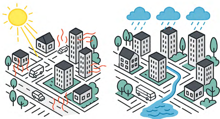
Figure 8. The image illustrates two major urban environmental challenges. Left: The urban heat island effect, where buildings and paved surfaces absorb and radiate heat, causing significantly higher temperatures in city areas compared to surrounding rural regions. Right: Urban flooding, resulting from intense rainfall and excessive soil sealing, such as surfaces with concrete and asphalt, which limits natural water absorption and increases runoff, leading to water accumulation and flood events.
